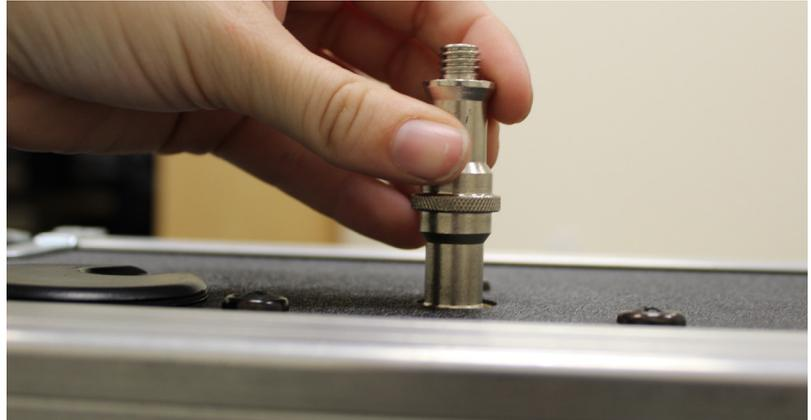
Take the threaded stud and screw into the top of the mirror case.
