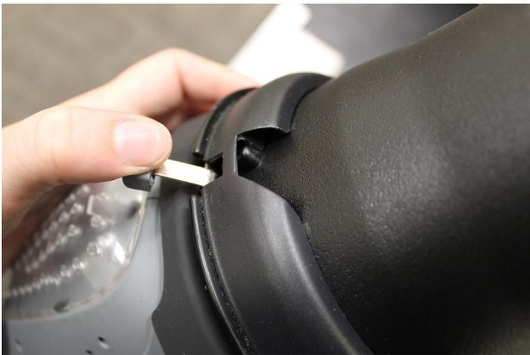
Remove the bulb case from the flash by pushing down on the switch and twisting the case. Place the reflector on by sliding into the slots and twisting.
